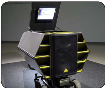
Audio System and Entry Hatch Open
