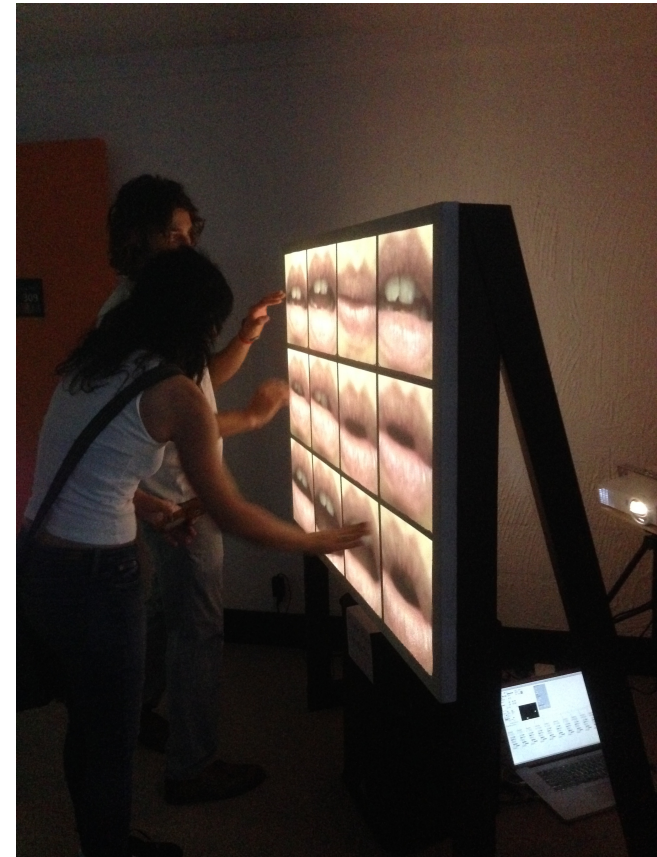
Figure 3: Two people interacting with the spandex fabric grid interface, and the projector and computer system behind the screen. ©Mathew Mosher
